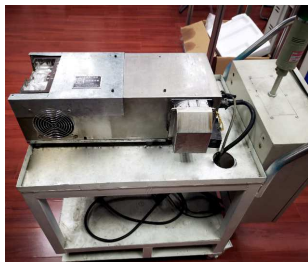
超声波浸焊设备 Ultrasonic dipping soldering equipment
