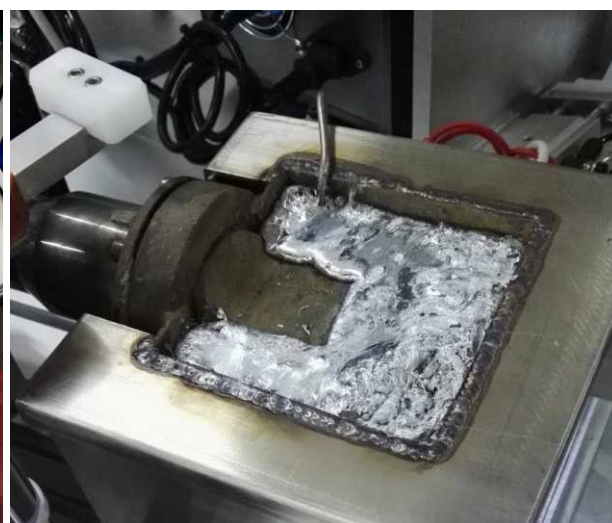
超声波浸焊设备 Ultrasonic dipping soldering equipment
