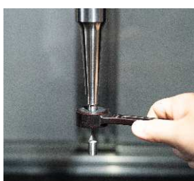
轴向对称拉压疲劳试验 Axial symmetric tension compression fatigue test
