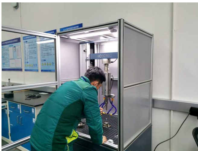
超声超高周疲劳试验 High cycle fatigue strength ultrasonic testing
