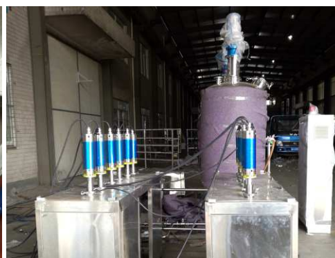
超声波石墨烯循环生产线 Ultrasonic graphene circulation production line
