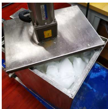
超声波石蜡乳化 Ultrasonic paraffin emulsification
