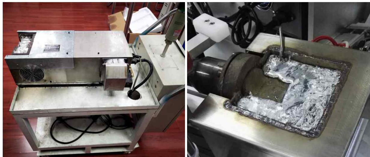
超声波浸焊设备 Ultrasonic dipping soldering equipment
